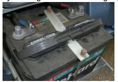
Deep cycle batteries always have bolt on connections with wing nuts, which distinguish them from common automotive batteries.
