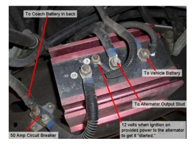
Here is a picture of a typical *battery isolator*:
