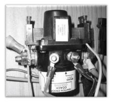
To "open" the relay, you reverse the connections to the coil, and this deflects the magnet away from the
