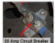
batteries, alternator and converter/charger can deliver tremendous current and circuit protection devices are a necessity.
